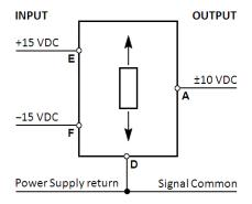
A through F: Connector pin assignments
